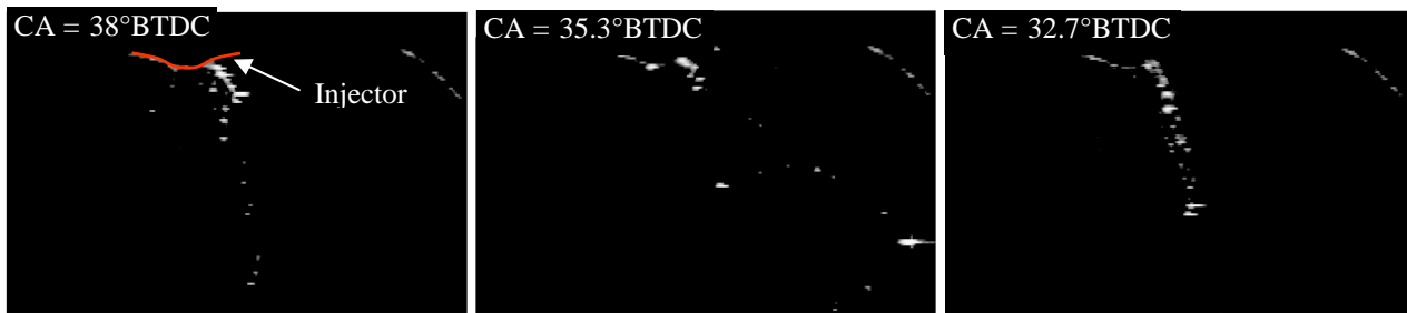
Figure 6 Large droplets after the end of injection.
