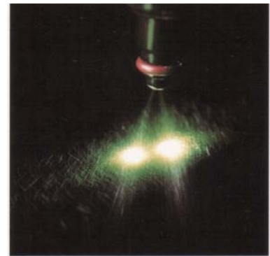
Gasoline fuel injector characterisation using output from FibreSheet
