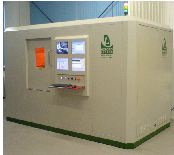
Fig.8. Oxford Lasers PicoLase 1000 picosecond laser micromachining system installed at MEC, Cardiff University
