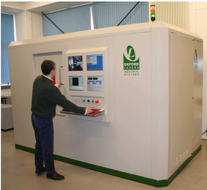
Figure 1 Oxford Lasers PicoLase 1000 picosecond laser micromachining system installed at MEC, Cardiff University
