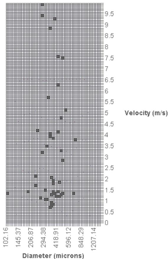
Figure 8. Size and Velocity Distribution Downstream of the Spacer Grid.
