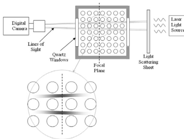
Figure 3. General Schematic of the Imaging System.
