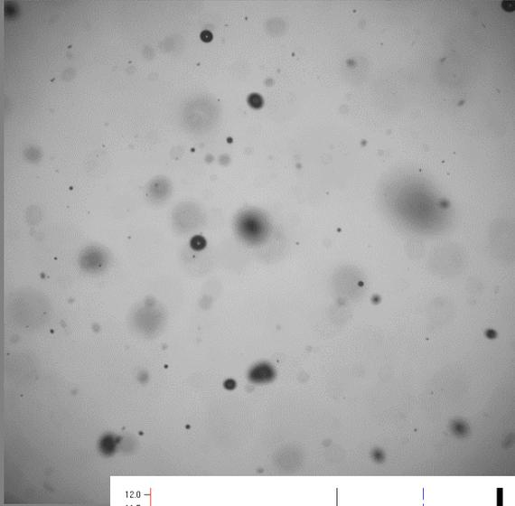
Visisize particle sizing software analyses the images of droplets in real-time and reports on their diameter. This means that you can see the droplet size distribution build up as the droplets pass the camera. Visisize reports all the measurements that you would expect from a best-in-class particle sizing instrument including:
