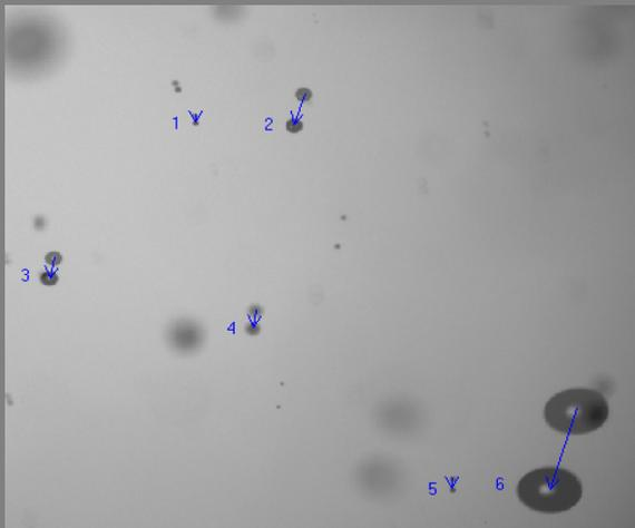
With the velocity function enabled, Visisize systems will simultaneously measure and report the particle size and velocity. This means that you can see what velocity different sizes of droplets are moving at. You can understand whether flow from your nozzle is dominated by fast or slow droplets, what direction they are travelling in, and what their mean diameter is.
